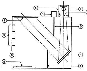
Fig. 1.—Schematic diagram of a compact pre-exposure unit.
