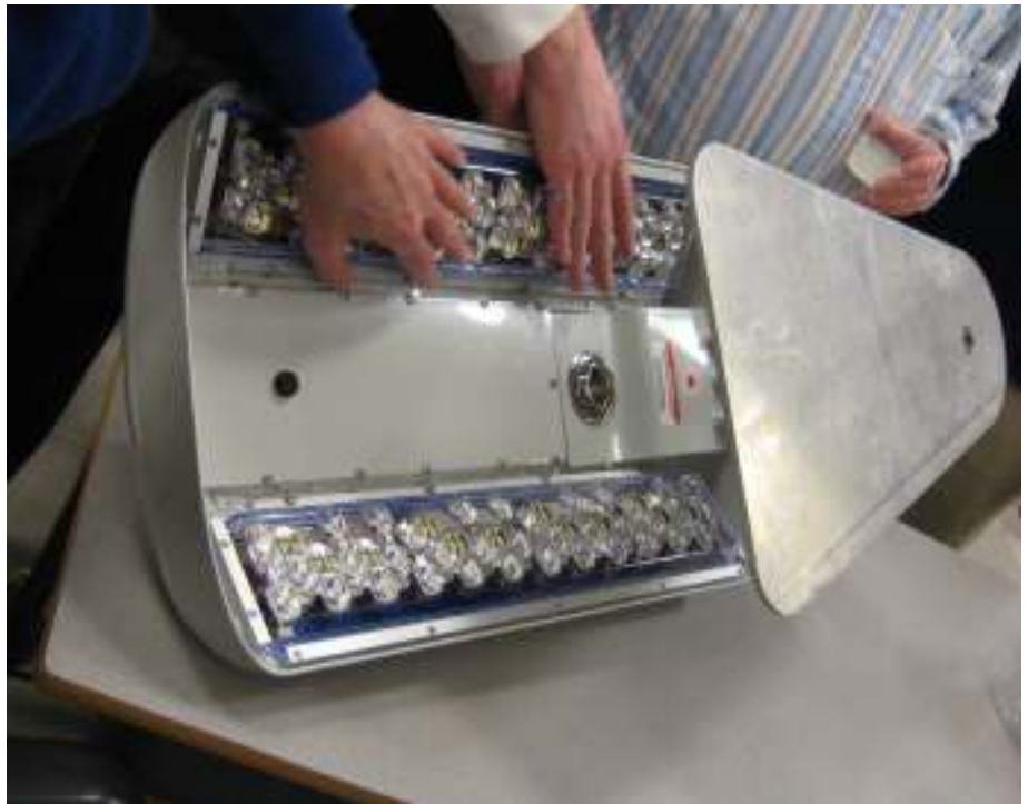
A "hands-on" view of the operational LED lighting fixture
