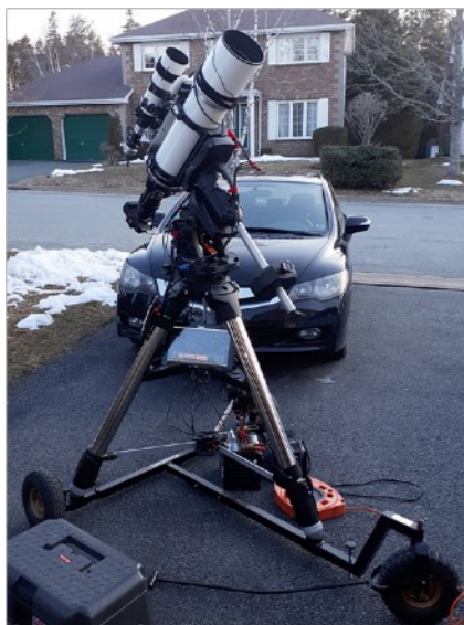
Figure 7 - My present setup. The Scope Buggy lets me wheel the scope from my garage to my driveway and be imaging within 20 minutes.
